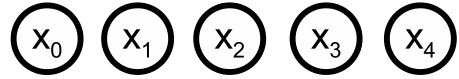
Figure 3: “True” structure for a 5-bit instance of onemax; no dependencies between variables
